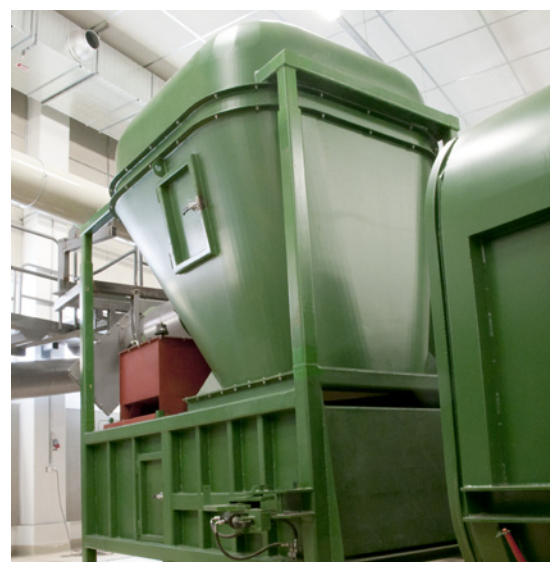
Above: Separator and compactor. Usage of compactors increases the amount of collected waste in the container and reduces the number of transports significantly.
